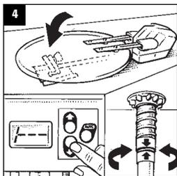
Before travelling, turn the mast until the black arrow stickers line up with each other to ensure the wheels rest on the wheel guide. Lower the dish by pressing the dish down button for at least 2 seconds. The dish will drive down and automatically stop at its lowest position when the down limit switch is triggered and the down limit symbol is displayed. Fasten the mast into position using the plastic spanner.
